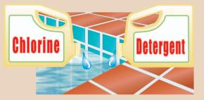
Chemicals added to the pool water tend to degrade cement-based grouts.
