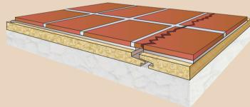
If a joint between wooden boards of a floating floor is not correctly located or fixed, it will be susceptible to highly localised movement which will crack the tile along
