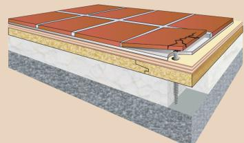
When a floating floor is over-boarded to add rigidity, the extra board has to be securely attached to the original boards. If nails are used, the constant movement of the floor can cause them to work loose, press on the underside of the tile and cause cracks to form. If the screws/nails used are too long they can bottom out on a rigid surface under the floating floor and create a column, over which tiles will crack.
