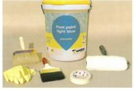
1 – Pool Paint is a 2 coat application. The first coat is applied by soft bristle brush and the second coat by sheepskin roller. Both coats must be applied on the same day.
