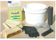
1 – Prepare 1 part of hydrochloric acid & 3 parts of water in a plastic bucket. Add water in the bucket first and then add the acid while stirring Be sure to wear gloves and eye protection.
